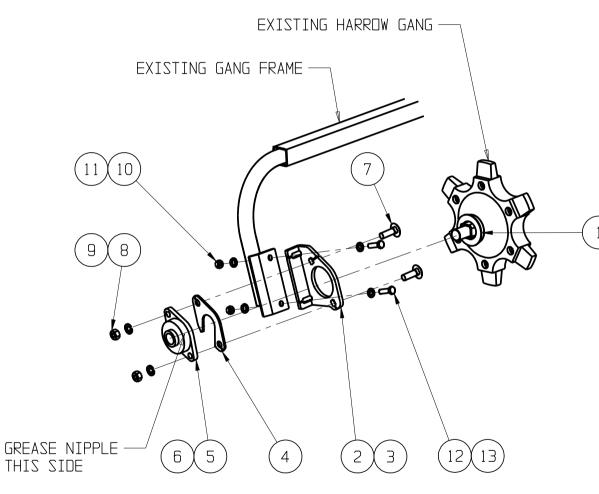
\* Grease bearings weekly. Do not over grease as seals may be damaged
